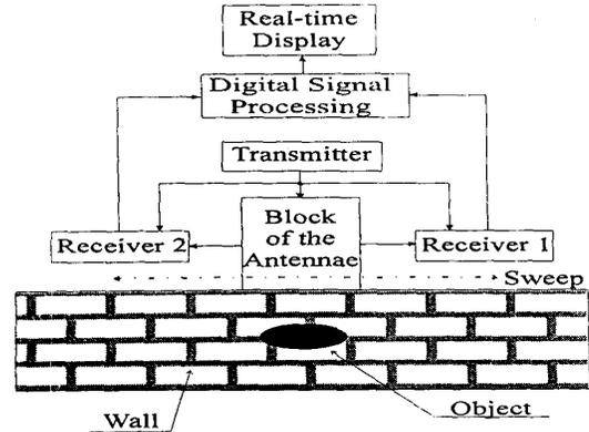
Fig. 2. Simplified Block Diagram of the Radar
