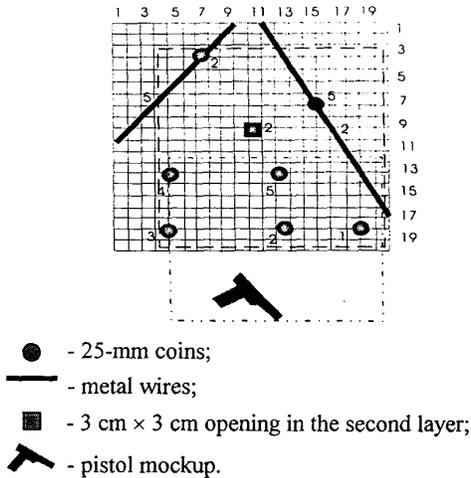
**Fig. 3. Arrangement of Objects in the Mockup Wall**
