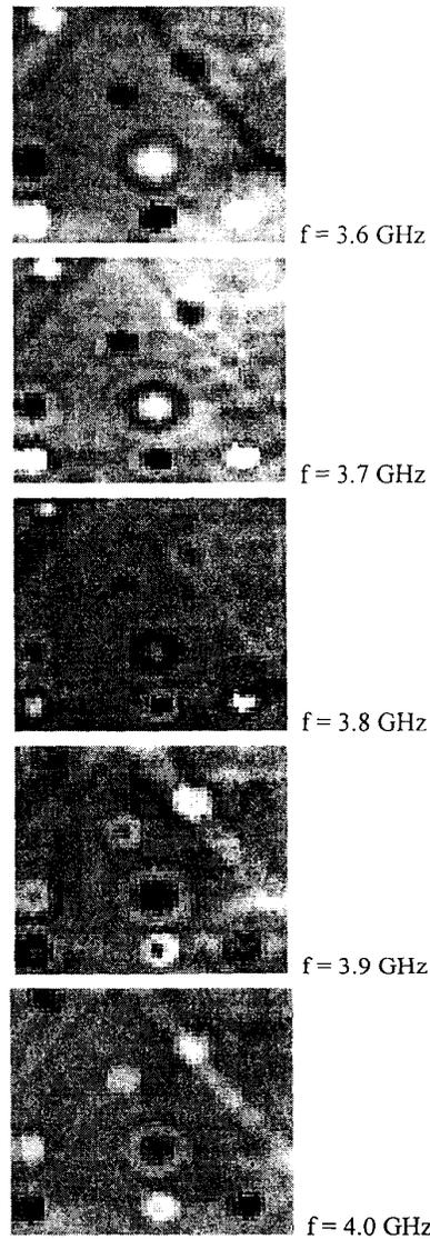
**Fig. 4. Radio Images Obtained by Five Frequency Channels by Using the Parallel Polarization of Received and Transmitted Signals**
