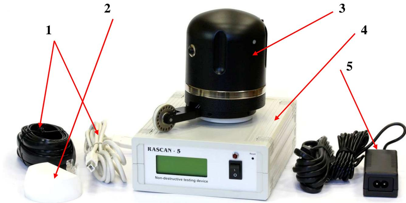
Fig. 1. Overall view of RASCAN-5 holographic subsurface radar: 1 – cables; 2 – antenna attachment for scanning in corners; 3 – radar head; 4 – control block; 5 – power supply unite.
