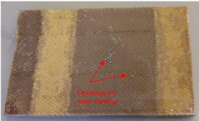
Fig. 6. View of the Sample 2. Two bright strips are cells that filled with polymer paste. Openings for water injection are indicated by arrows.
