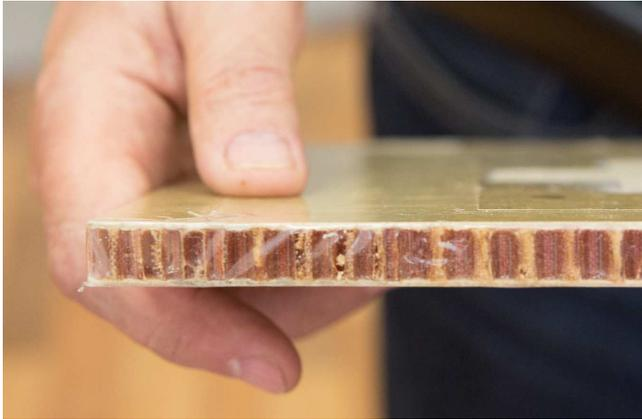
Fig. 3. View of the honeycomb strip from the butt-end of the composite panel.
