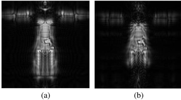
Figure 6: Microwave images of the pistol and body reconstructed for a single-frequency. (a) Mono-static case, (b) multi-static case.
