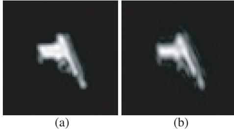
Figure 3: Microwave image of the pistol reconstructed for a single-frequency. (a) Mono-static case, (b) multi-static case.
