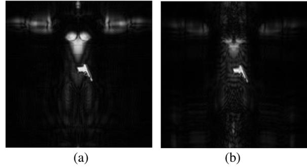
Figure 7: Microwave images of the pistol and body reconstructed for a wide-band hologram. (a) Mono-static case, (b) multi-static case.
