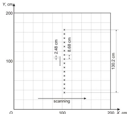
Figure 1: Multi-static antenna configuration.
