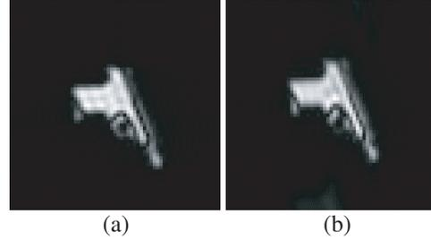
Figure 4: Microwave image of the pistol reconstructed for a wide-band hologram. (a) Mono-static case, (b) multi-static case.
