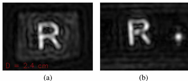
Figure 3. Comparison of the radar images obtained by adaptive scanning for around 1 minute (a) and by traditional way for around 9 minutes (b).
