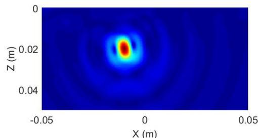
Figure 4: Reconstructed microwave image for phantom from Fig. 2 for probing frequency band of 10 GHz.
