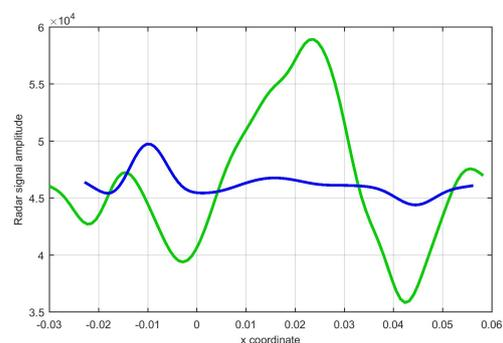
Figure 7: Experimental results for the phantom without (blue line), and with metallic inclusion (green line).
