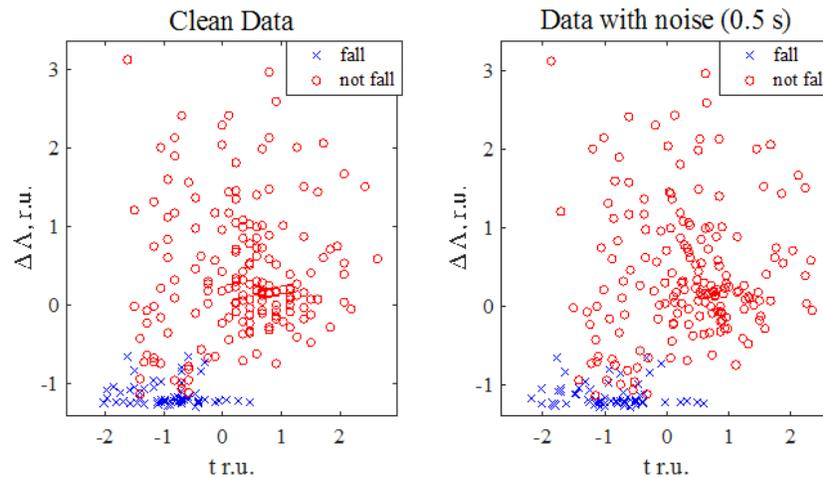
Figure 3. Scatter plot of obtained values of classification parameters (probing frequency = 3, 8 GHz).
