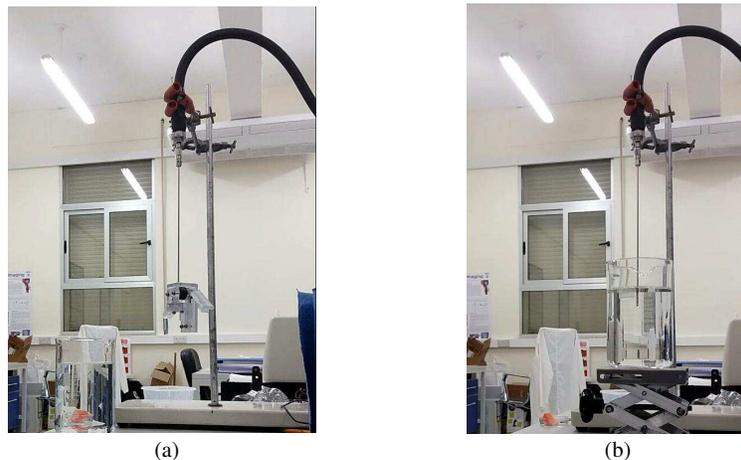
Figure 3: Calibration procedure: (a) by using the calibration short; (b) by using the water.
