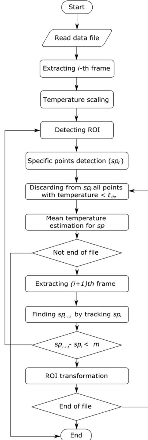
Figure 3. Flow-chart of the algorithm for thermal video processing
