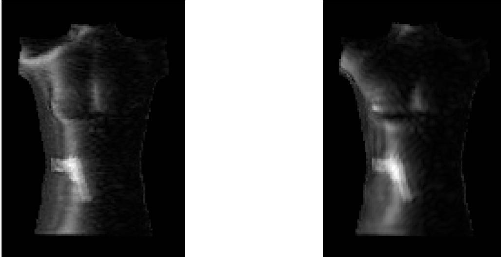
Figure 6. Radar images obtained with dense antenna array (left) and sparse antenna array (right). Sparse antenna array has reduced number of antenna elements by a factor of 7.
