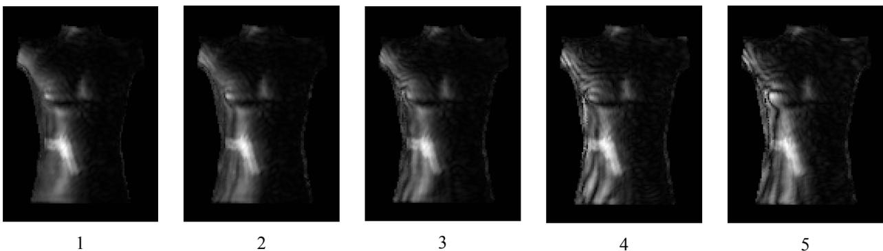
Figure 7. Radar images obtained for the sparse antenna arrays having various numbers of transmitters and receivers.
