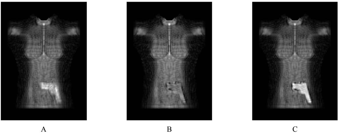
Figure 12. The radar images obtained by using the surface of the clothing. The single-frequency case.
