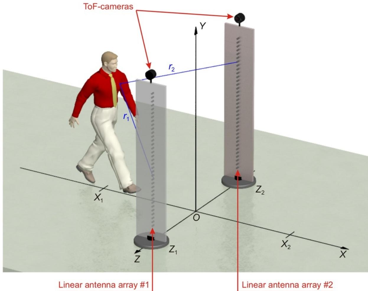
Figure 1. A possible geometry of the microwave screening system implemented as ISAR.
