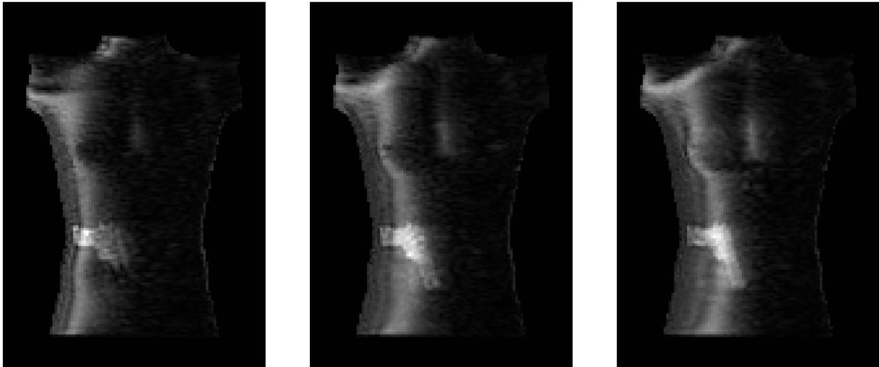
Figure 8. Radar images calculated for the different lengths of synthetic aperture: 1 m (left), 1.5 m (middle), 2 m (right).
