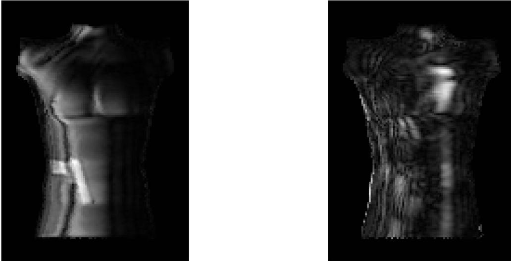
Figure 4. Calculating the radar image: with precise trajectory information available (left), with a rough estimation of the trajectory (right).
