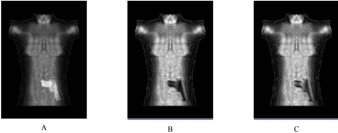
Figure 10. The radar images obtained with precise knowledge of the surface. The wide-band case.
