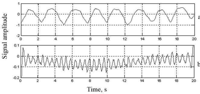
Fig.2. Reconstructed breathing and heart beat signals of the examinee corresponding to range-frequency matrices from Fig.1.
