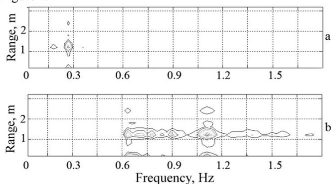
Fig.1. Range-frequency matrix for the examinee at 1.5 m range: a) (upper panel): before breathing harmonics rejection; b) (lower panel) after breathing harmonics rejection.
