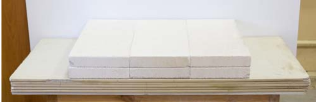
Figure 3: Foam concrete slabs and plaster sheets used in experiments.
