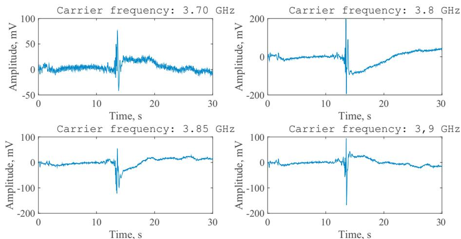
Figure 2: Charts of signal records of backward falling pattern at 4 different carrier frequencies (I quadrature).
