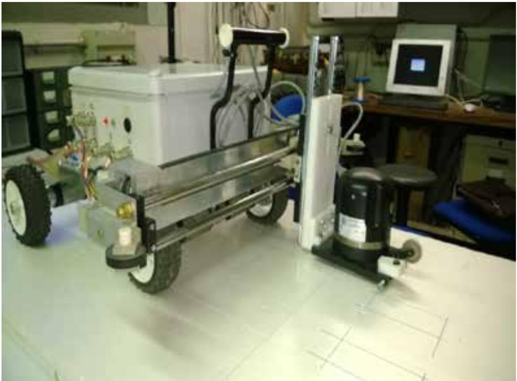
**Fig. 2.** Robotic scanner with a 4 GHz (RASCAN-4/4000) holographic radar during the thermal insulating panels inspection. It is possible to see on the bottom left corner the two panels of 18 mm thick one over the other with minimal air gap.
