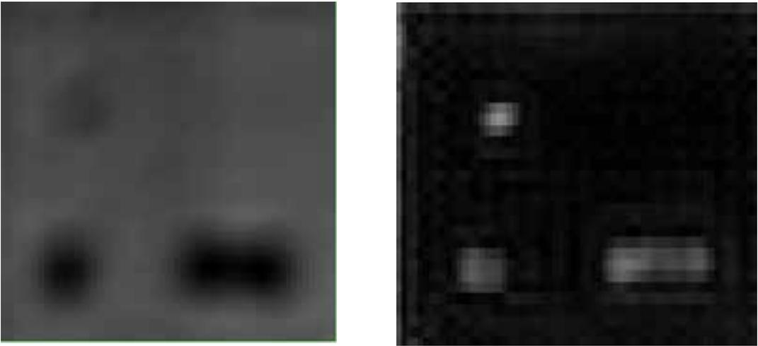
**Fig. 5.** Comparison of holographic radar imaging in parallel polarization of the four targets shown in Fig. 1: 3.9 GHz (left), 6.7 GHz (right).
