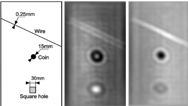
Fig. 5. Map of the foreign objects in a stack of plaster sheets (left), real (center) and imaginary (right) parts of the parameter  $S_{21}$
