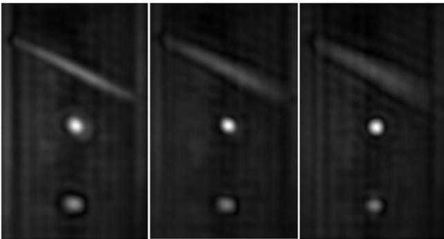
Fig. 6. Reconstructed radar images focused on the wire (left), on the square hole (center) and on the coin (right)
