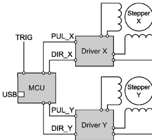
Fig. 2. Stepper motor control diagram
