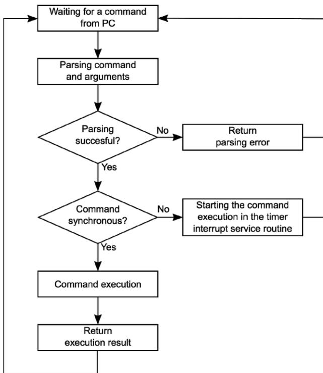
Fig. 4. The main execution cycle in the embedded software
