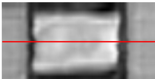
Figure 5. Holographic image of the phantom #1 (air gapping excluded).
