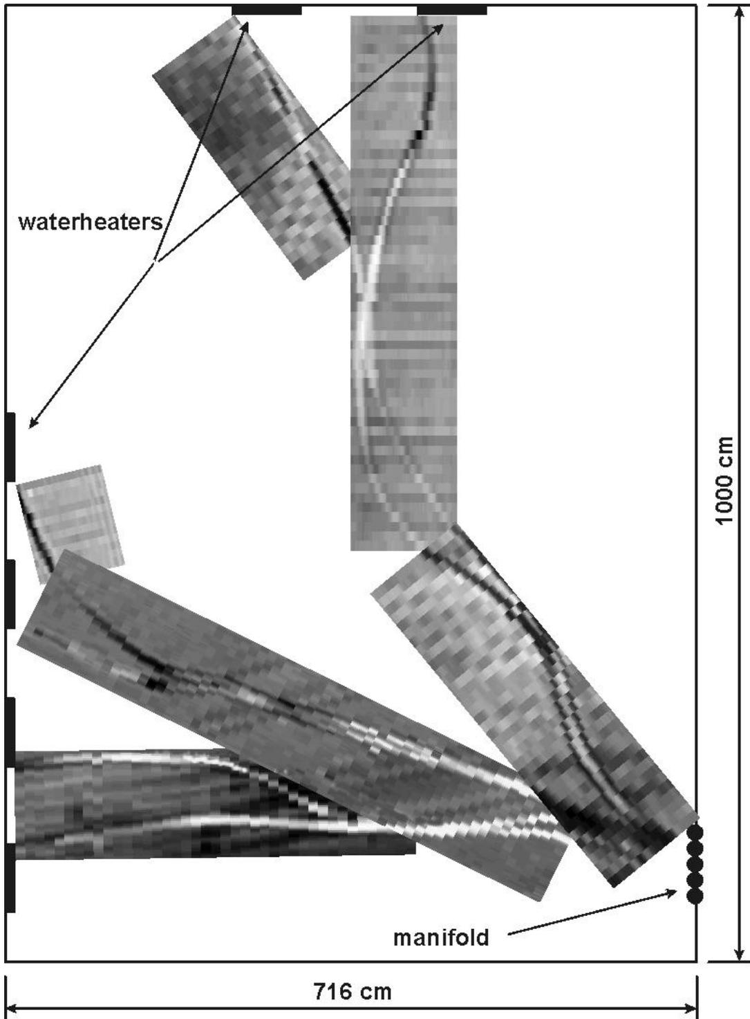
Figure 4: Radio-image of plastic tubes under a concrete floor covering.
