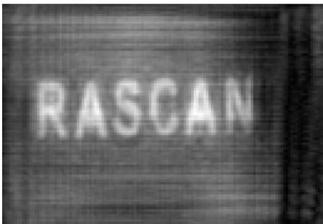
Figure 13. A reconstructed image of aluminum foil letters behind a plaster sheet.
