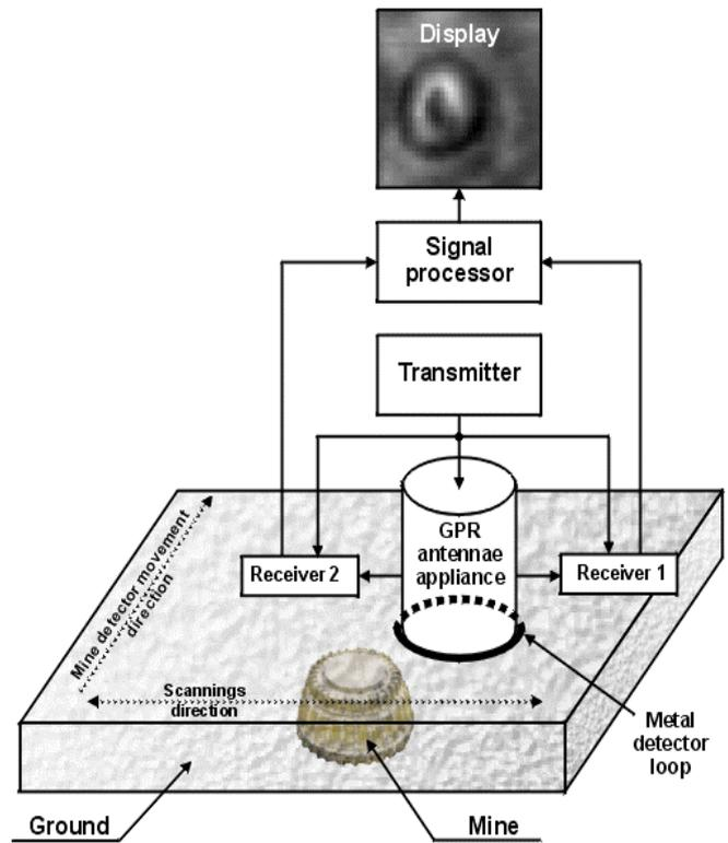
Figure 2: Block diagram of MiRascan radar with metal detector.
