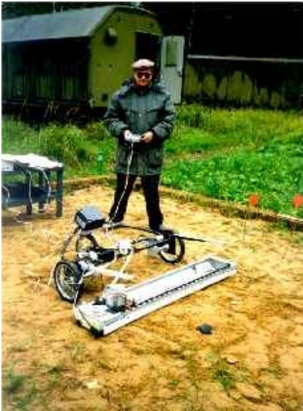
Figure 1: Two-channel MiRascan mine detection system.
