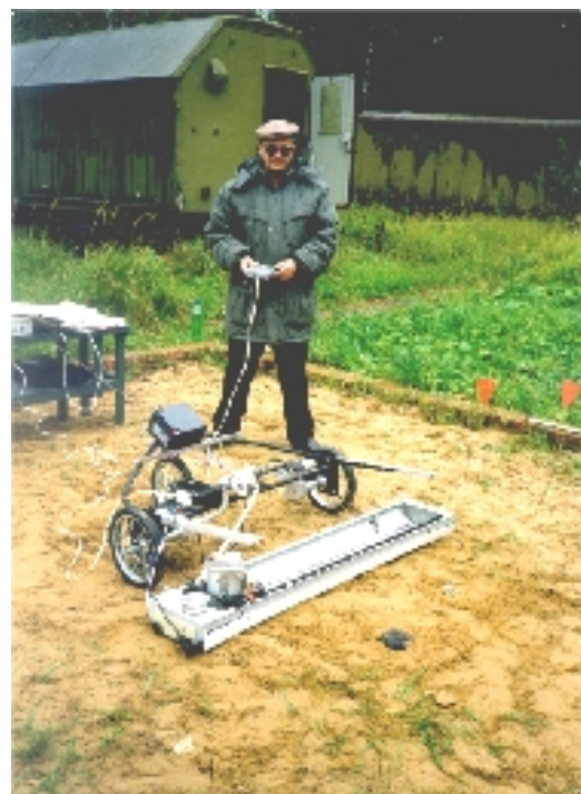
Fig. 7. Two-channel MiRascan mine detection system.
