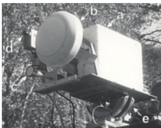
Fig. 2. Experimental installation includes radiometer (a), radiometer's antenna (b), noise generator with horn antenna (c), TV camera (d) and two-dimensional scanning device (e)
