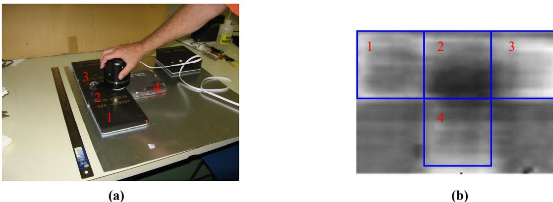
**Figure 10:** (a) Process of Scanning sample shuttle tiles: **Tile 1** was bonded with a layer of contamination (hand lotion) on the aluminum; **Tile 2** was bonded properly; **Tile 3** was bonded on the left half only; **Tile 4** was bonded with only a spot of RTV. (b) RASCAN image for the sample tiles: darker areas represent proper bonding, and the lighter area shows subnominal bonding (lateral resolution ~ 1 cm).
