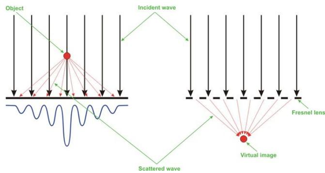
Figure 7: Recording and Reconstruction of microwave hologram.
