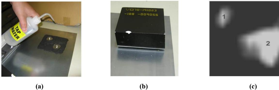
**Figure 11:** (a) A thin layer of RTV was applied to the Aluminum plate. Two spots were left intentionally without RTV to create subnominal bonding: upper left part (1) has an air pocket; the lower right part (2) has water drops between the tile and the substrate; (b) A 6 x 6 x 2 inch tile was bonded on the place; (c) A RASCAN image of tile shows the subnominal bond (light part in upper left) and subnominal bond filled with water droplets (lighter part in lower right).
