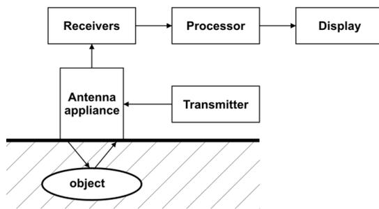
Figure 8: Block Diagram of RASCAN.
