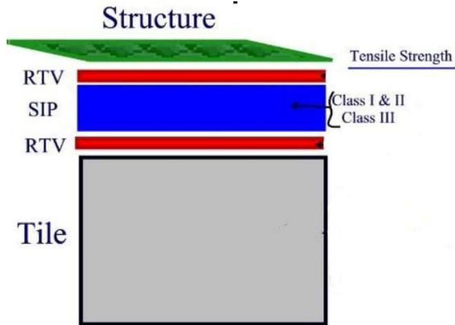
Figure 3: Cross Section of Tile Adhesion with Tensile Strength
