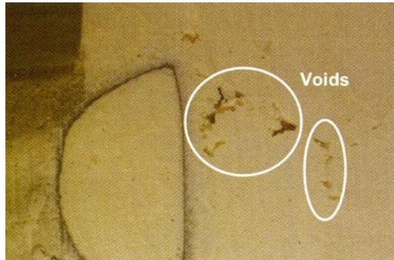
*Figure 2. Close-up of voids in the external tank insulating foam<sup>2</sup>.*
