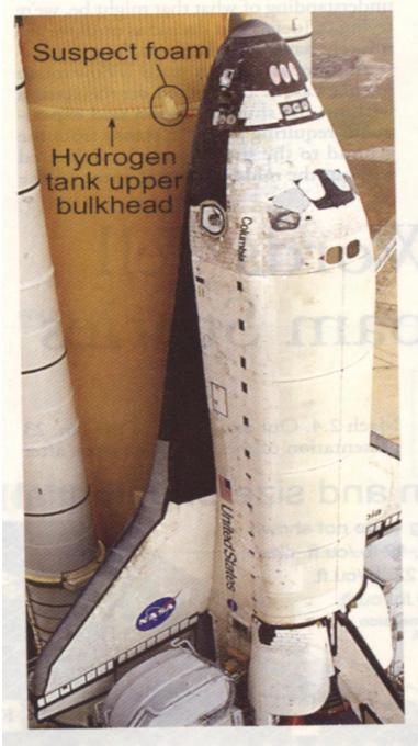
*Figure 1. Suspect flaws on the external hydrogen tank coating<sup>1</sup>.*
