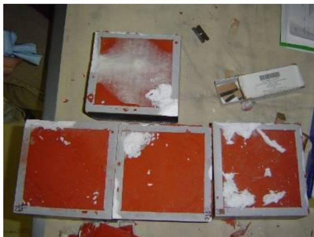
Figure 5: Nominal SIP to Tile Bond Condition
