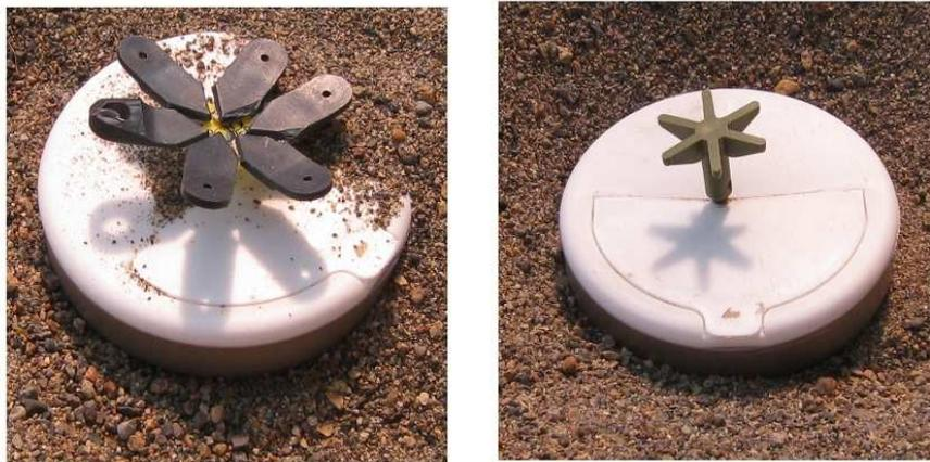
Figure 2: LEFT) target A with big trigger, filled with granulated sugar (dielectric constant from 2.5 to 3.2) RIGHT) target B with small trigger.
