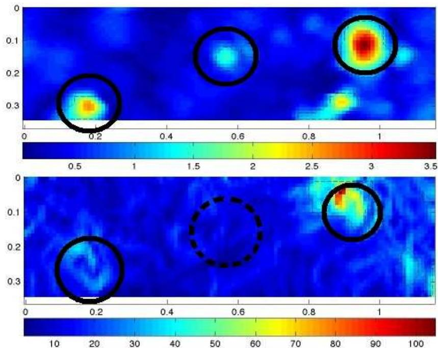
Figure 7: Top) Scanning in contact with ground Bottom) Scanning with air gap LEFT) target C MIDDLE) target B RIGHT) target A.
