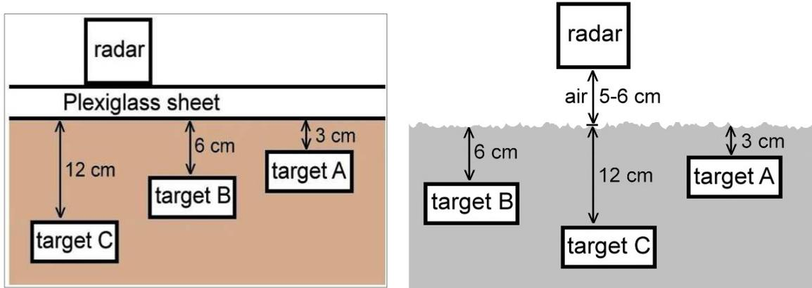
Figure 6: Section view of the layout of Italian experiment.
