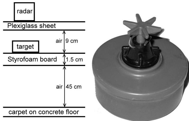
Figure 4: LEFT) Layout of experiment from USA RIGHT) View of the PMA-2 mine simulant.
