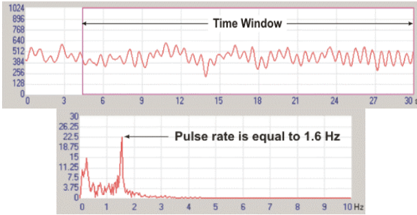
Figure 6. Pulse record of the examinee and its signal spectrum.. Breath delay equals to about one minute.
