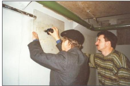
**Operators with the RASCAN-4 radar during the wall examination**
