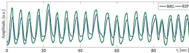
Fig. 5. Peak-to-peak synchronization of RIP and BRL signals.
