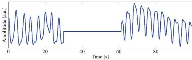
Fig. 4. The BRL signal. The signal oriented normally on the left side. The rejected artefact interval are in the center. The signal inverted on the right side.
