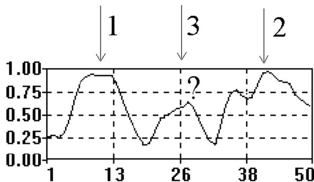
Fig. 5. The amplitude of radar signal measured in the upper part of the vault along line A-A in Fig. 4
