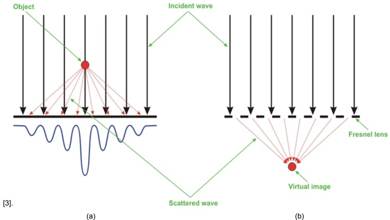
Fig. 2. Recording (a) and reconstruction (b) of a hologram
