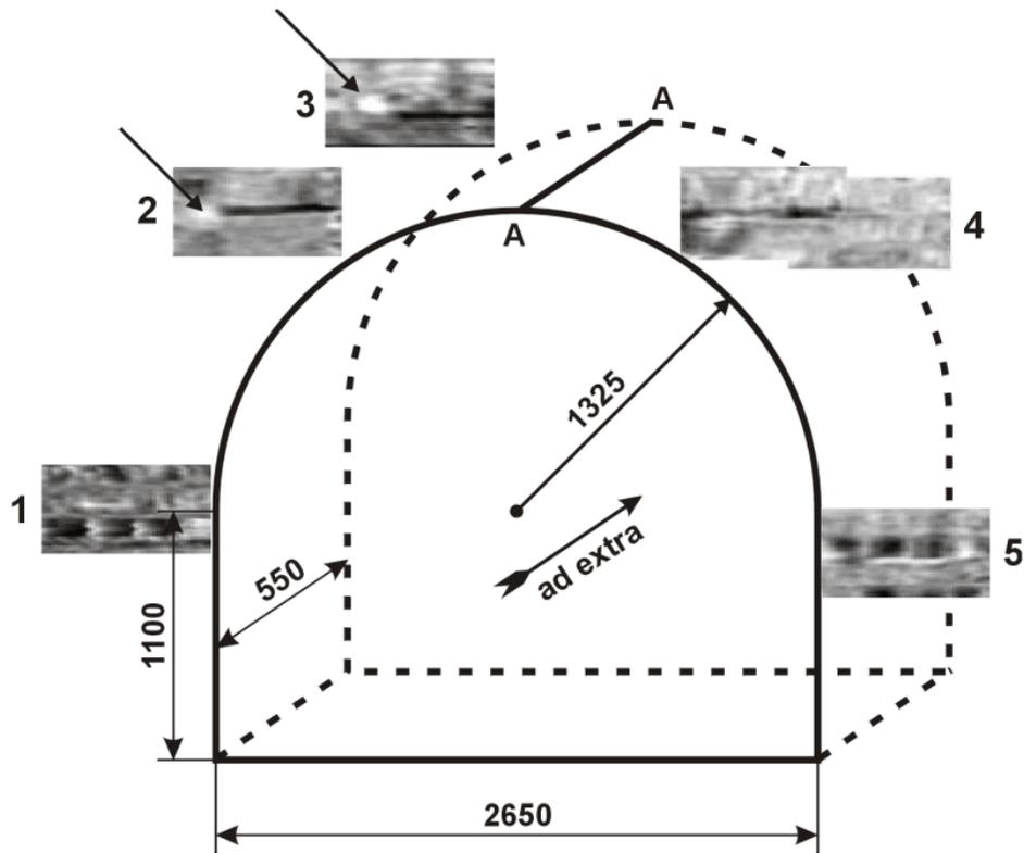
Fig. 4. Geometrical parameters of the investigated arch and the results of radar sounding. The arch dimensions are presented in centimeters
