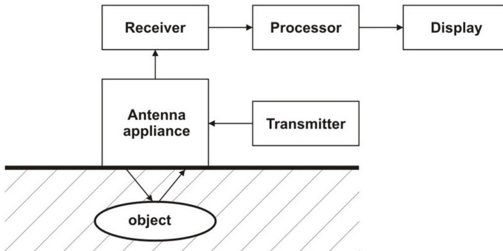
Fig. 1. Block diagram of subsurface radar system
