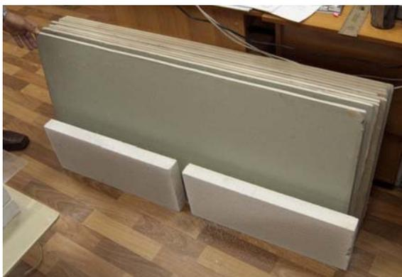
Figure 4. Photograph of foam bricks and plaster sheets that were used in experiments.
