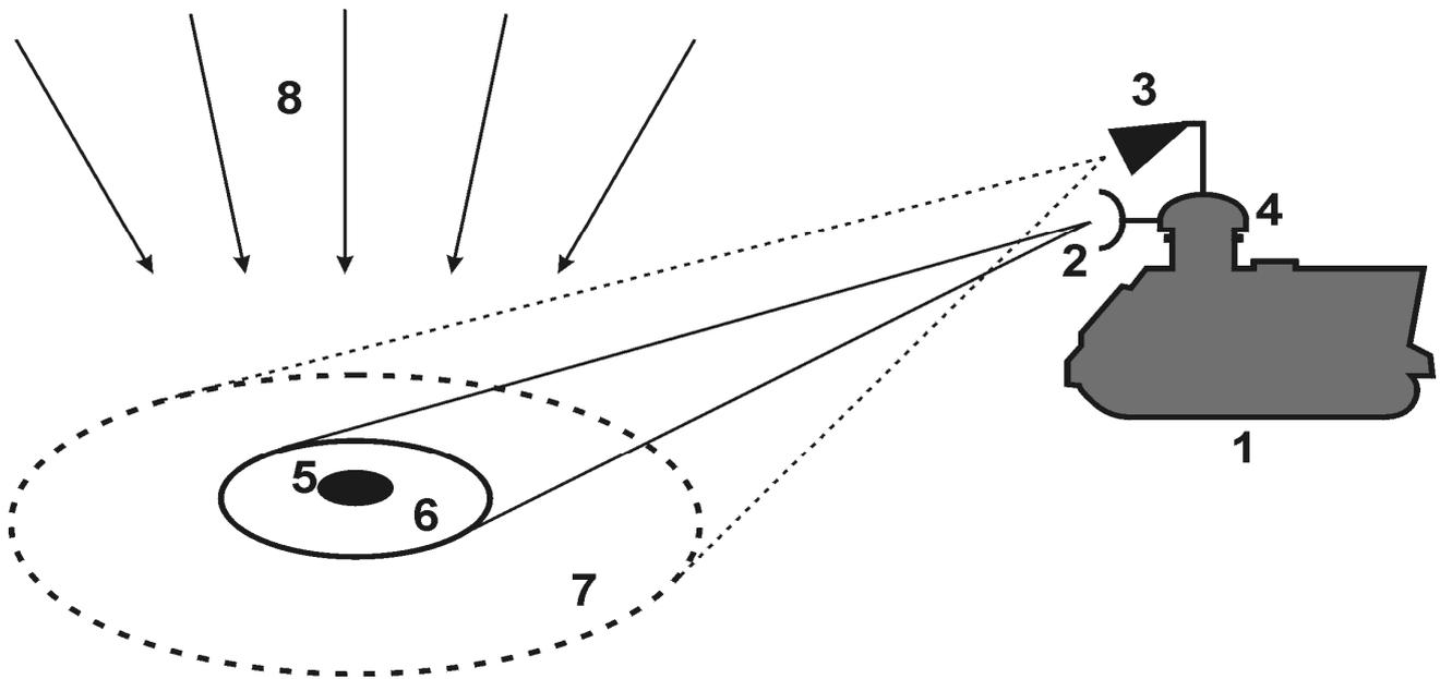
Figure 1. Principal arrangement of passive/active radiometer
