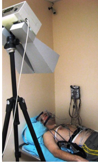
Figure 1. Scheme of the experiment on simultaneous registration of BRL and PSG data during sleep.
