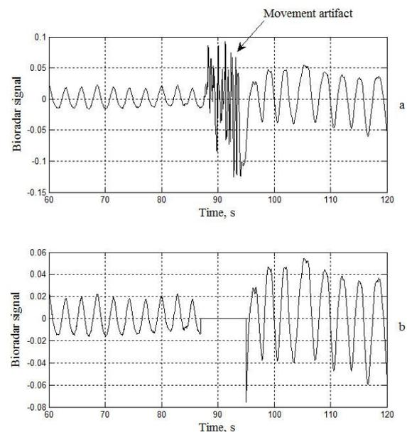
Fig.2. Bioradar signal before (a) and after (b) movement artifact extraction
