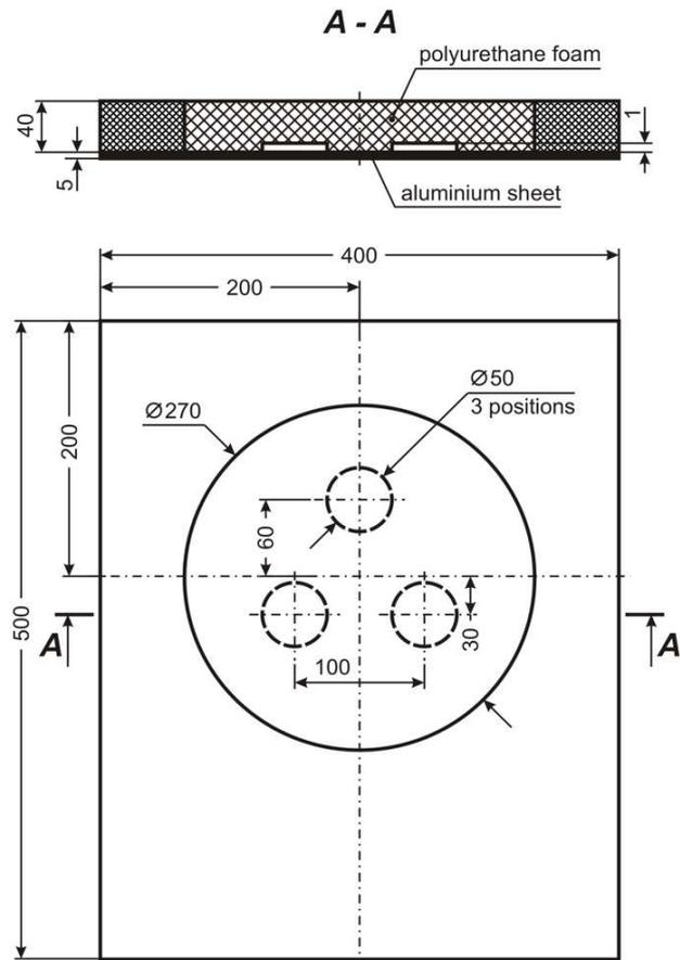
Fig. 3. Draft of the polyurethane insulation sample
