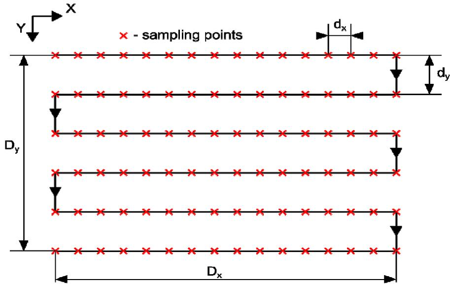
Fig. 2. Diagram of a sample scanning
