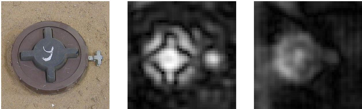
Figure 7. PMN-2 anti-personnel mine: photo (left), radar image of the mine on the surface from the distance of 9 cm (middle), radar image of the mine when it is buried by 2 cm in sand from the distance of 1 cm from the surface (right). The sounding frequency is equal to 6.7 GHz.
