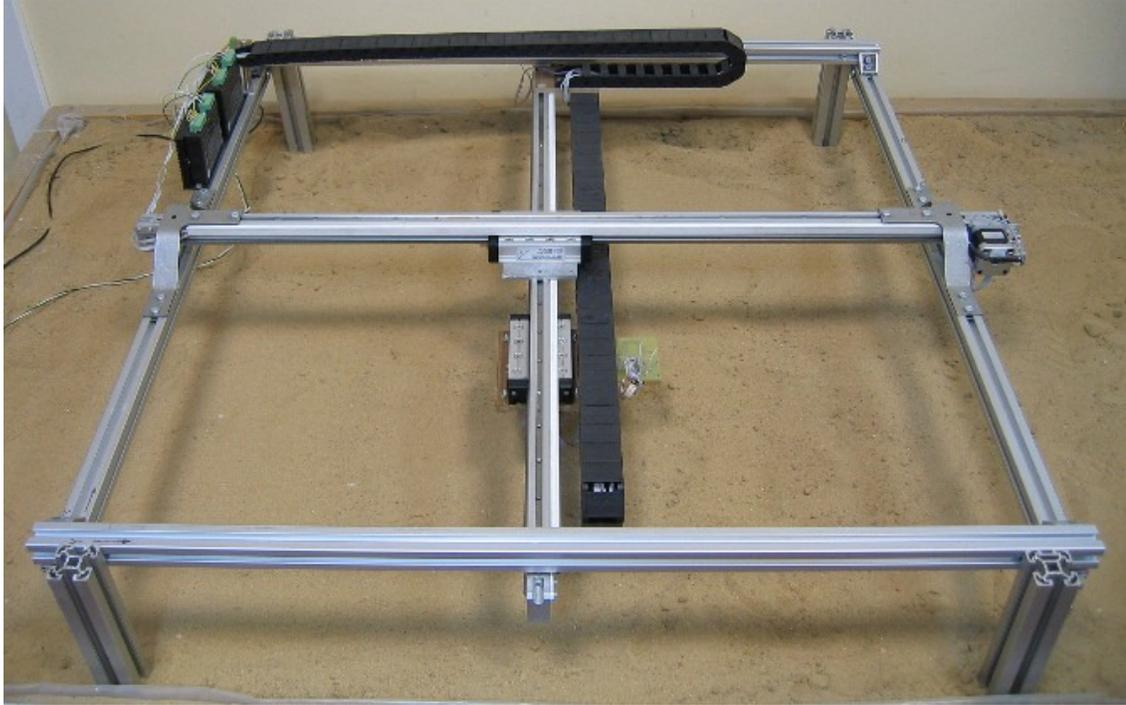
Figure 2. Electro-mechanical scanner for hologram acquisition.
