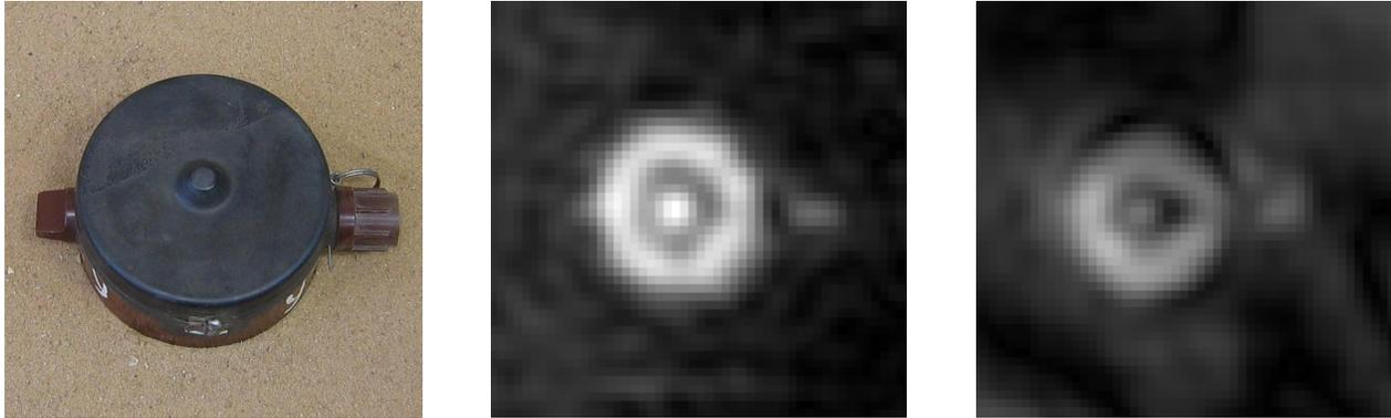
Figure 8. MC-3 anti-personnel mine: photo (left), radar image of the mine on the surface from the distance of 6 cm (middle), radar image of the mine buried by 2 cm in sand from the distance of 2 cm from the surface (right). The sounding frequency is equal to 6.4 GHz.
