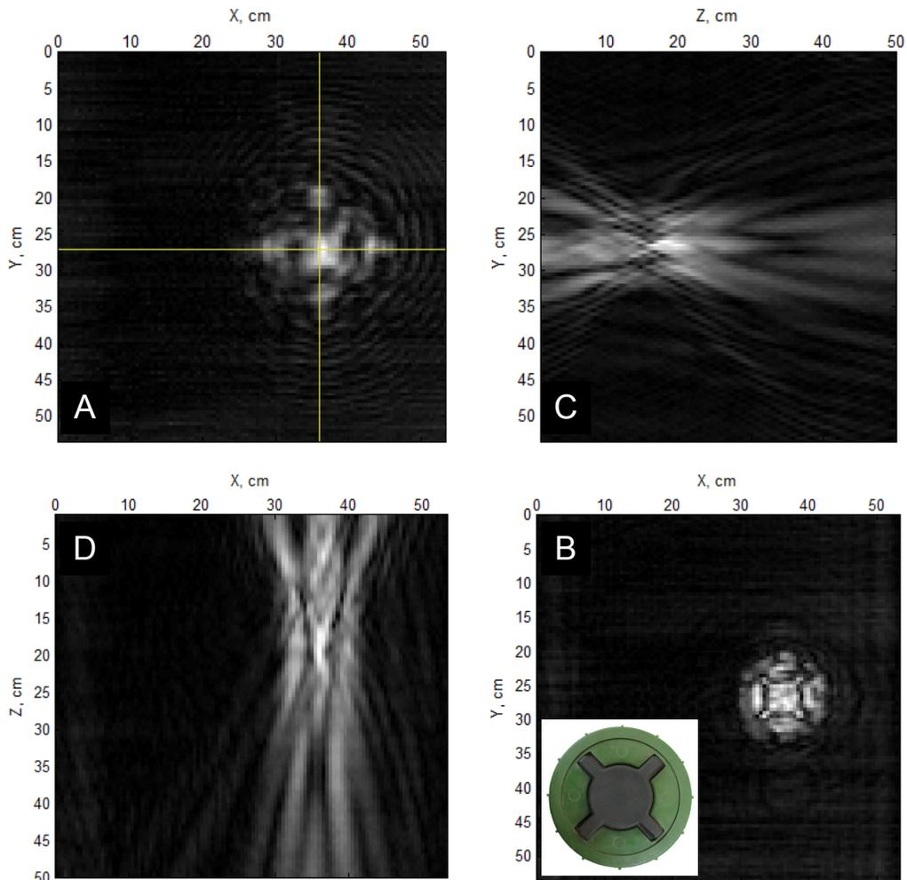
Figure 6. Cuts of reconstructed volume: *A* – amplitude hologram acquired at the interface with intersecting lines being projections of *YZ*- and *XZ*-cut, *B* – the plane of best focus with a photo of the test object, *C* – *YZ*-cut of reconstructed volume, *D* – *XZ*-cut of reconstructed volume.
