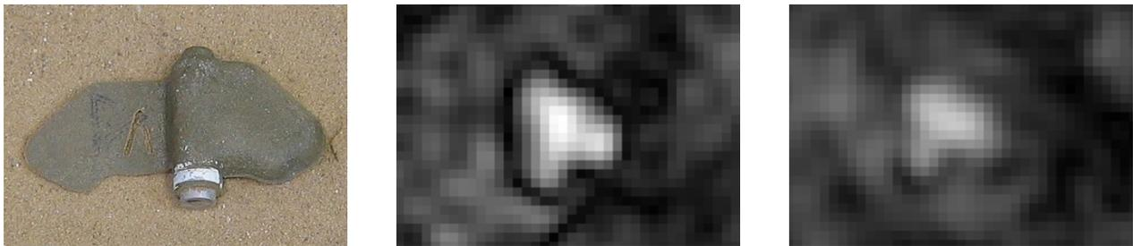
Figure 9. PFM-1 anti-personnel mine: photo (left), radar image of the mine on the surface from the distance of 9 cm (middle), radar image of the mine buried by 1 cm in sand from the distance of 3 cm from the surface (right). The sounding frequency is equal to 6.4 GHz.
