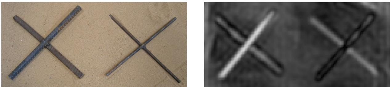
Figure 10. Metal reinforcement bars with the diameters 16 and 8 mm: photo (left), radar image of the bars buried by 2 cm in sand from the distance of 1 cm from the surface (right).
