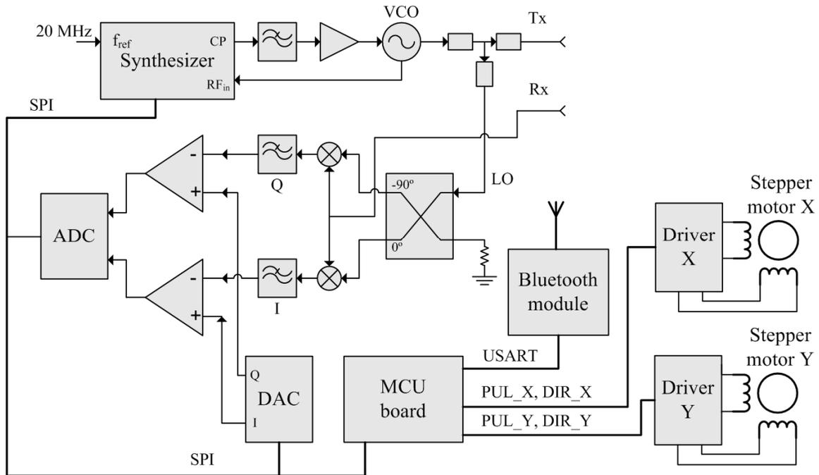
Figure 3. Principal diagram of the data acquisition system with the radar and scanner.
