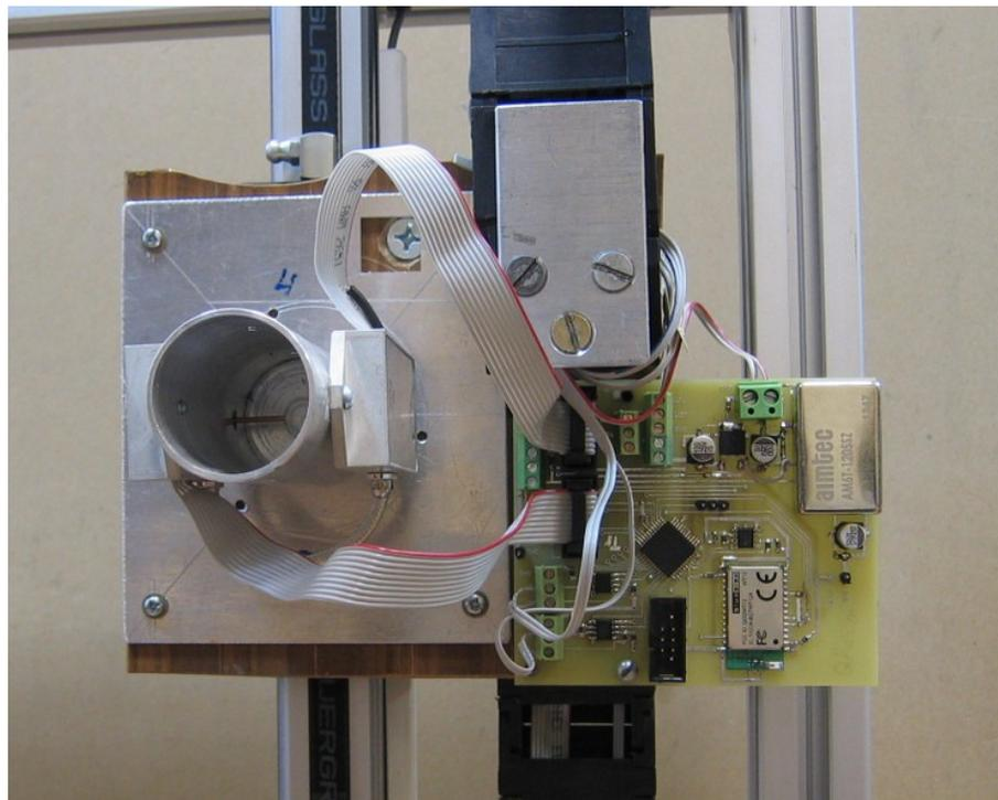
Figure 4. Continuous wave radar for the frequency band 6.4 – 6.8 GHz.
