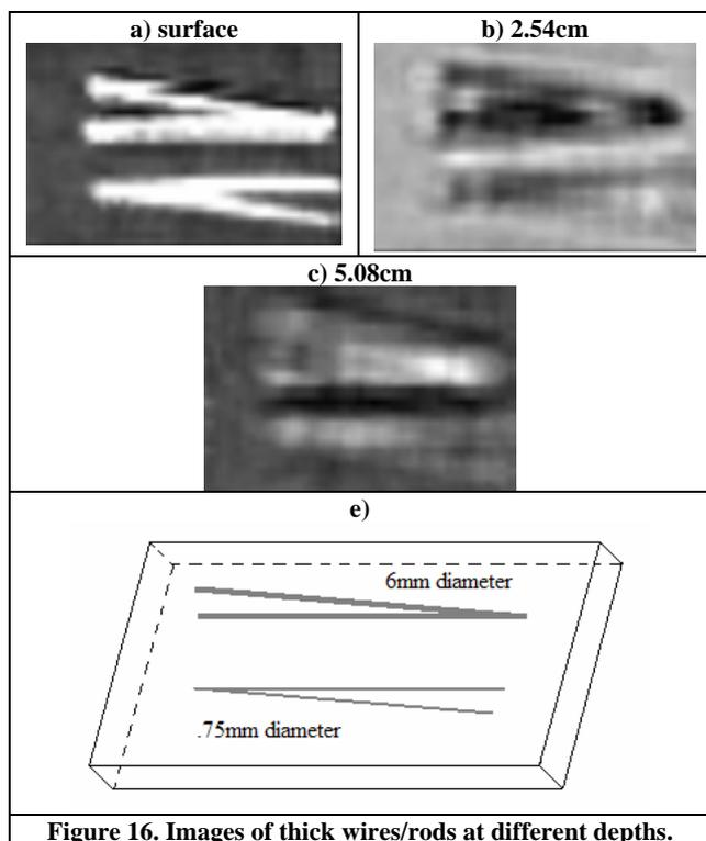
Figure 16. Images of thick wires/rods at different depths.
