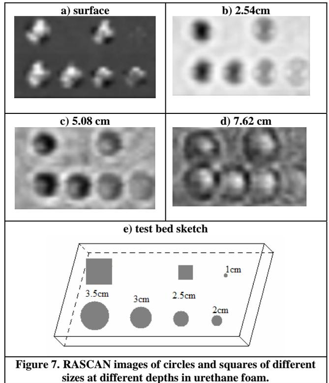
The array of coins was placed on a piece of urethane foam, which was then scanned repeatedly at increasing depths (0, 2.54, 5.08, and 7.62cm) beneath other layers of foam. The array consisted of a line of decreasing-diameter circular coins, with a parallel line of square coins (if available) with side lengths equal to the diameter of the adjacent circular coin. Square coins of side length 3.5 and 2.5cm were found. Also, placed in the upper right corner of the bed, was a 1cm aluminum tack head.
