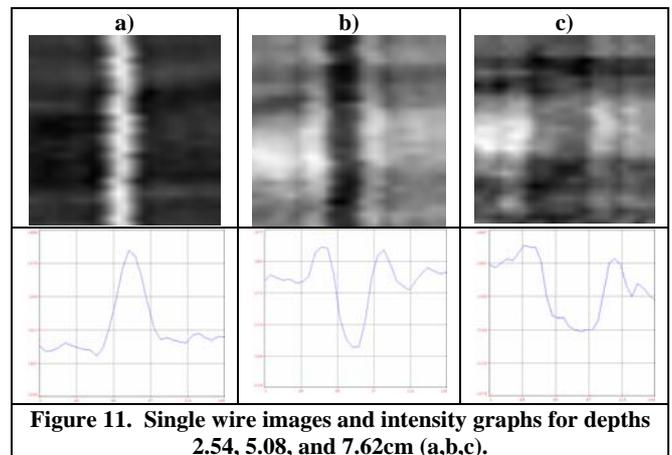
**Figure 11. Single wire images and intensity graphs for depths 2.54, 5.08, and 7.62cm (a,b,c).**
