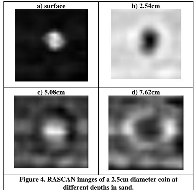
Figure 4. RASCAN images of a 2.5cm diameter coin at different depths in sand.
