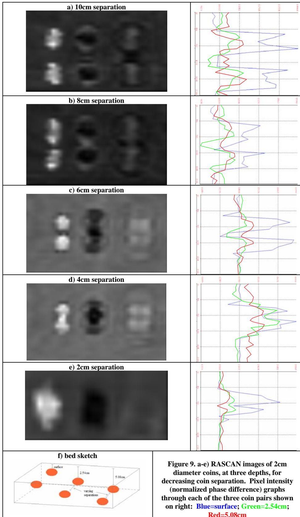
Thus, applying the strict Rayleigh Criterion to these images, the resolution is at least 2cm at depths down to at least 5.08cm for these 2cm diameter circular targets. Note that these images illustrate also the common pattern for RASCAN images as described above for the other tests; the deeper a target, the lower the intensity of its Airy spot, and the more pronounced the diffraction rings.
