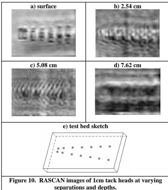
**Figure 10. RASCAN images of 1cm tack heads at varying separations and depths.**
