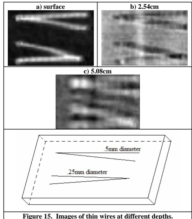
**Figure 15. Images of thin wires at different depths.**
