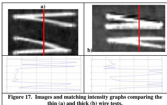
Figure 17. Images and matching intensity graphs comparing the thin (a) and thick (b) wire tests.
