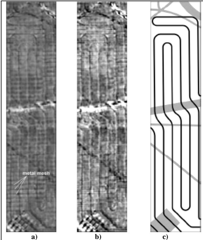
**Figure 2. From [2]. a) Raw RASCAN image of sub-floor; b) same image after Fourier domain filtering to remove metal mesh, c) layout of pipes and communication cables based on radar results.**
