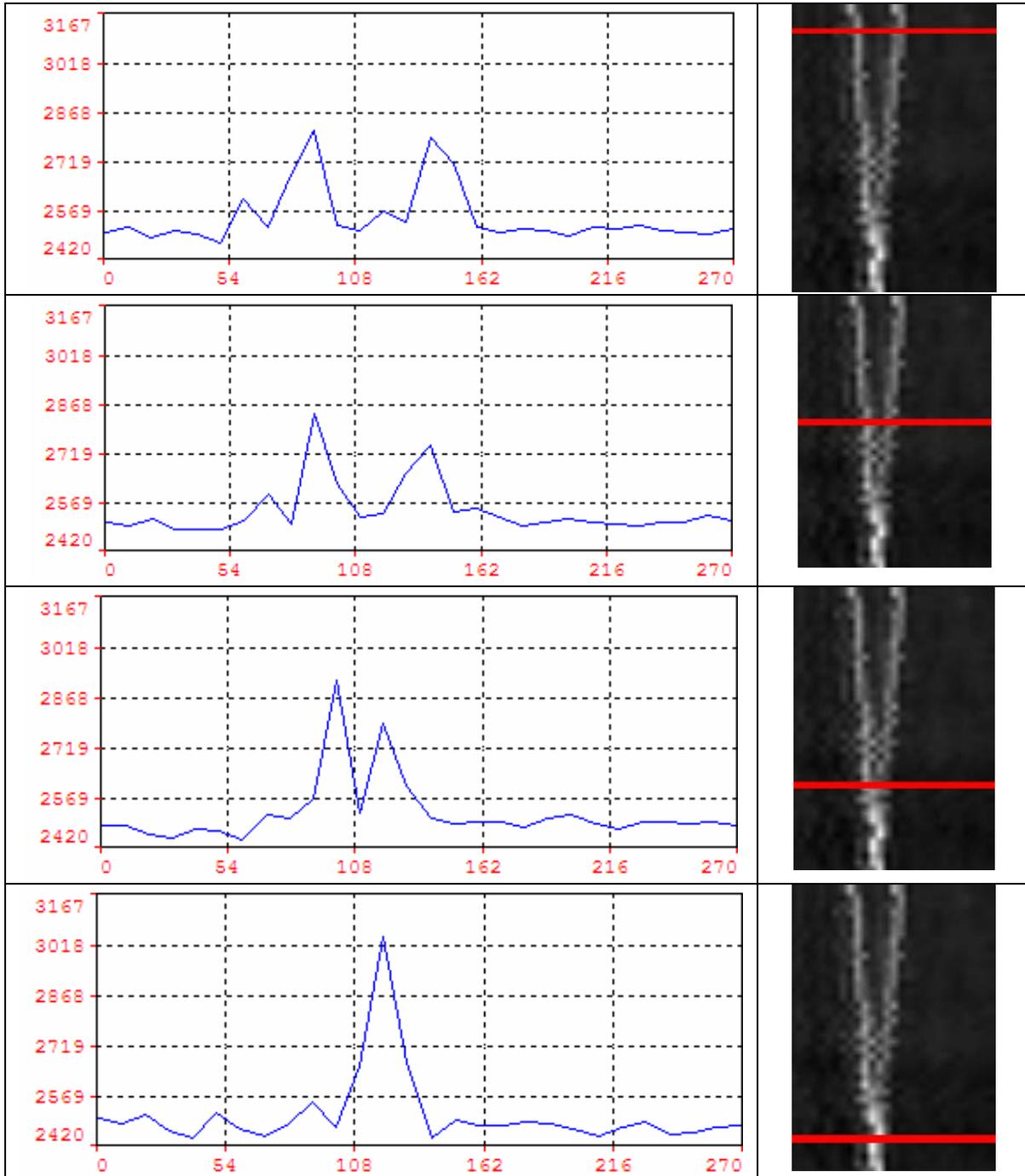
**Figure 12. Intensity graphs and images showing peak-to-peak separation, and merging of peaks. The red line on the image shows the row of pixels graphed on the left.**
