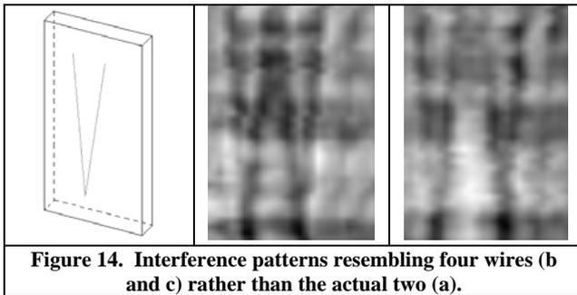
**Figure 14. Interference patterns resembling four wires (b and c) rather than the actual two (a).**
