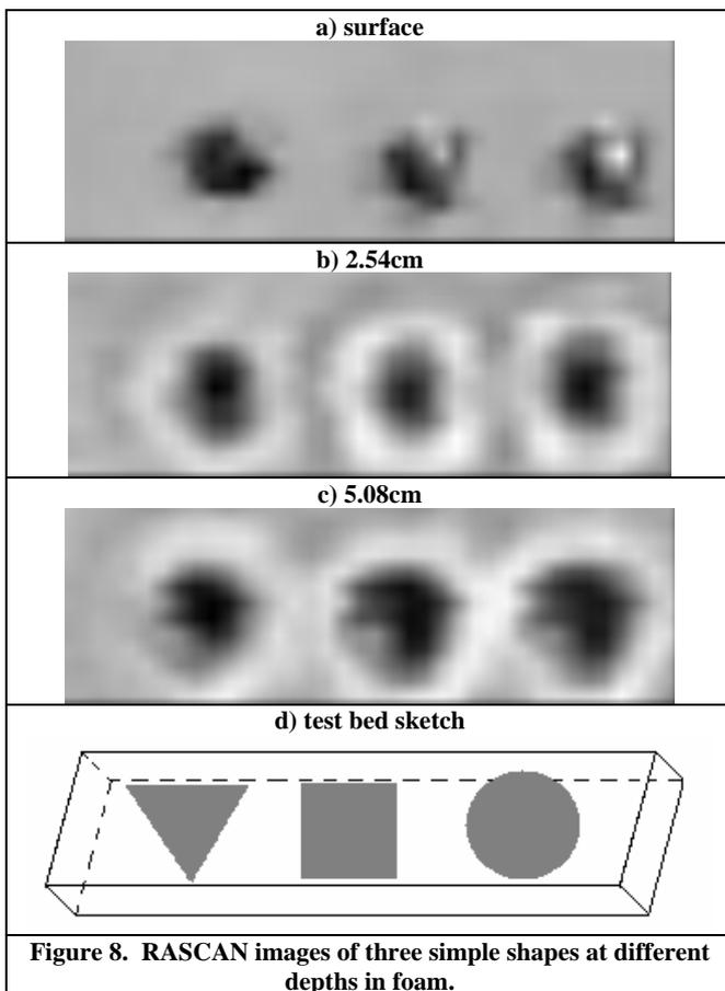
Figure 8. RASCAN images of three simple shapes at different depths in foam.
