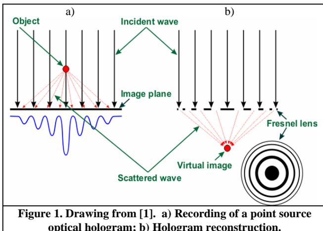
**Figure 1. Drawing from [1]. a) Recording of a point source optical hologram; b) Hologram reconstruction.**
