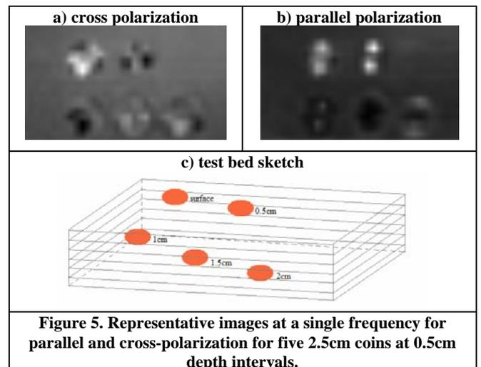
Figure 5. Representative images at a single frequency for parallel and cross-polarization for five 2.5cm coins at 0.5cm depth intervals.
