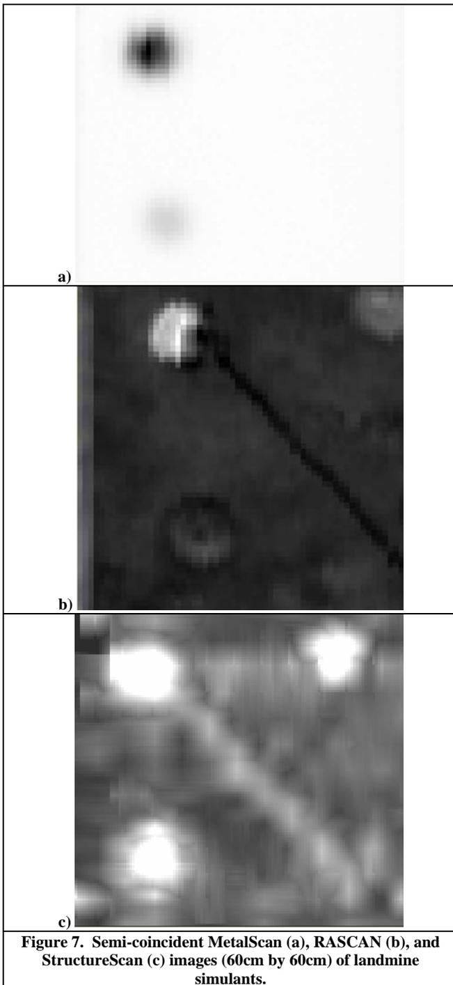
RASCAN produces ten simultaneous images at five frequencies for each of two different receiver polarizations (Fig. 8). As Fig. 8 shows, certain frequencies and/or polarizations provide clearer images due to greater phase differences – which cannot be predicted a-priori. The MultiScan software addresses this by providing a utility to construct a video in which the ten images smoothly transform into one another.
