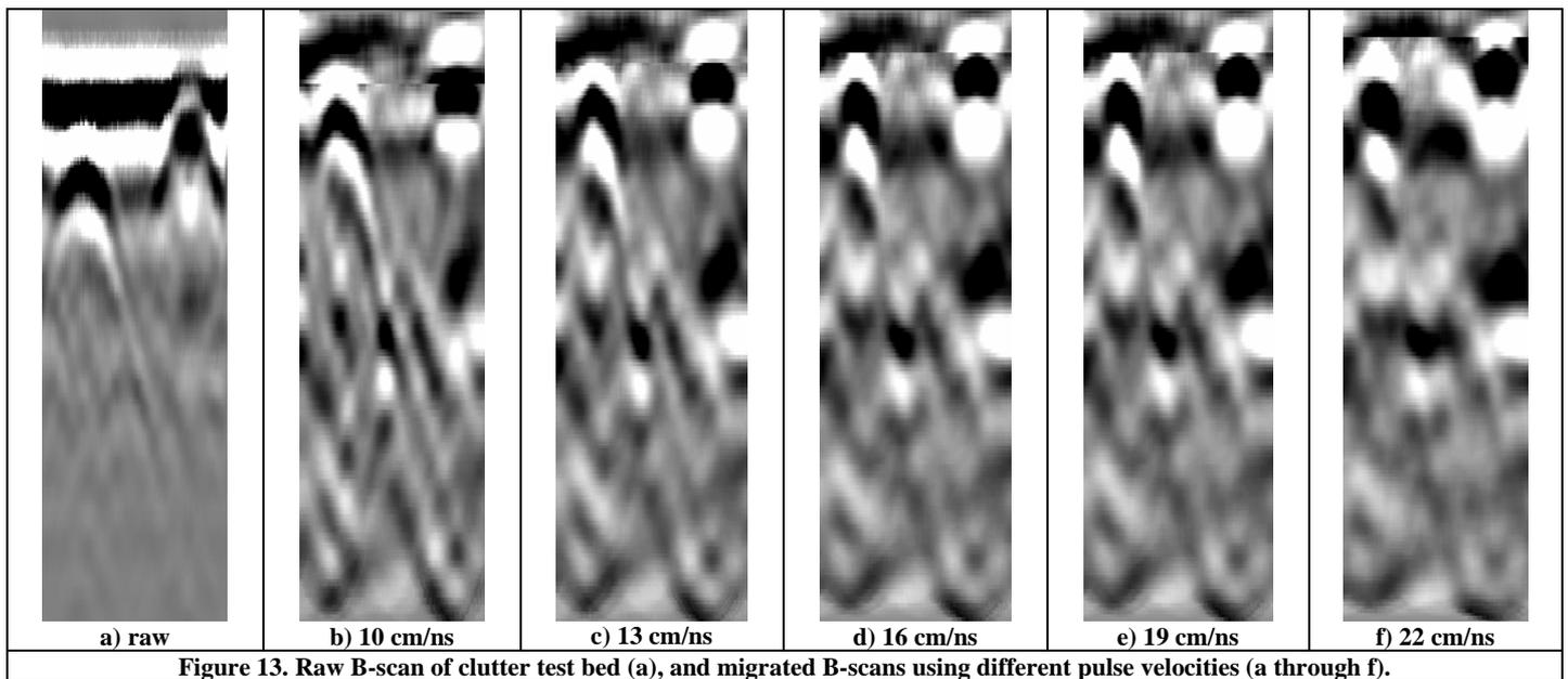
Figure 13. Raw B-scan of clutter test bed (a), and migrated B-scans using different pulse velocities (a through f).
