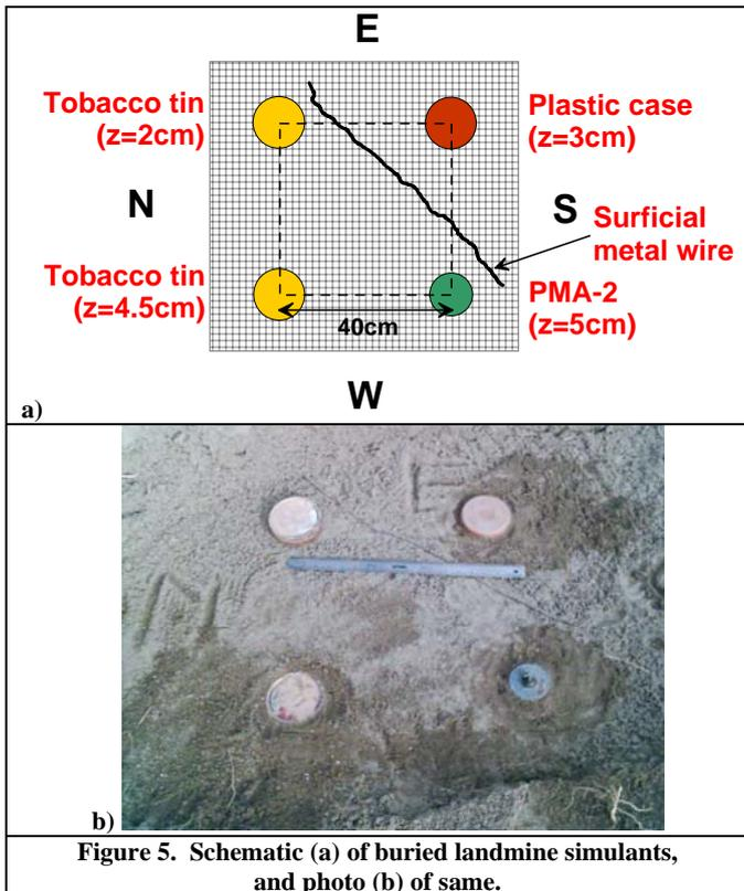
Figure 5. Schematic (a) of buried landmine simulants, and photo (b) of same.
