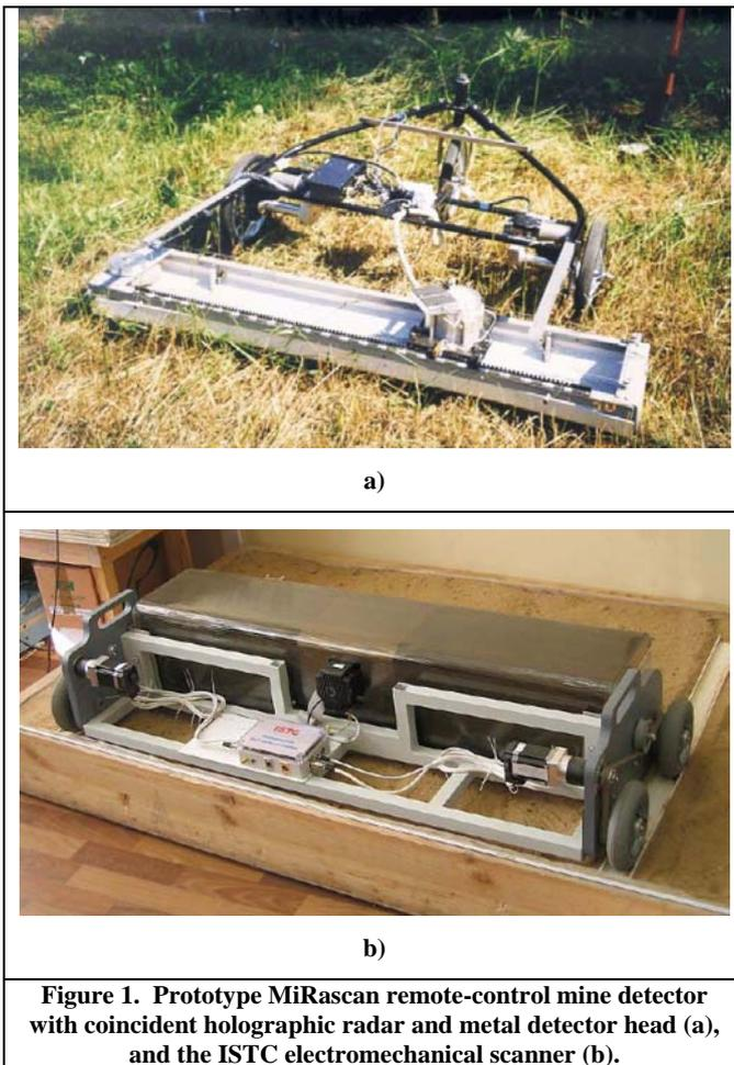
**Figure 1. Prototype MiRascan remote-control mine detector with coincident holographic radar and metal detector head (a), and the ISTC electromechanical scanner (b).**
