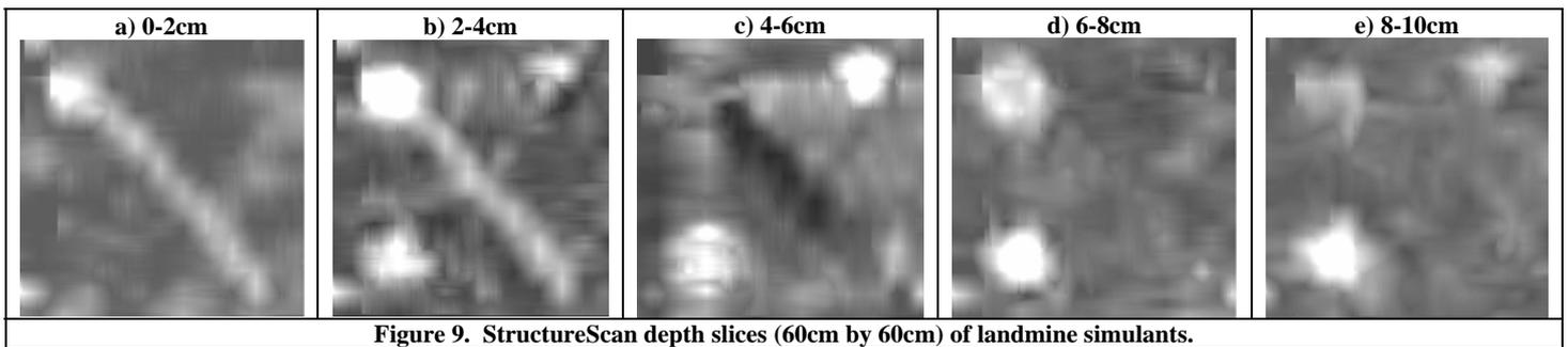
Figure 9. StructureScan depth slices (60cm by 60cm) of landmine simulants.
