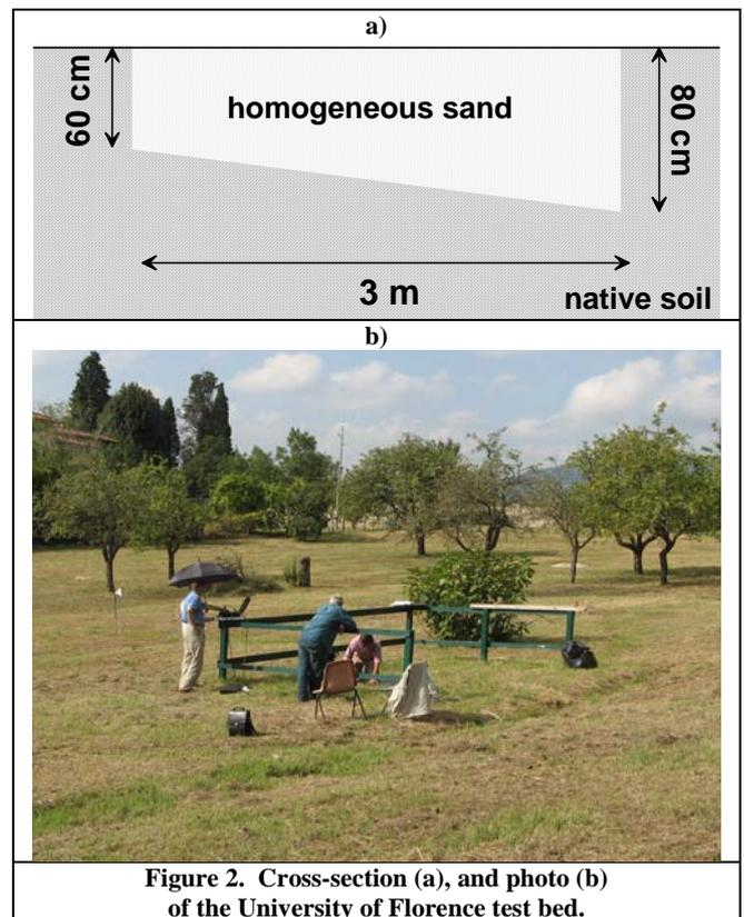
**Figure 2. Cross-section (a), and photo (b) of the University of Florence test bed.**
