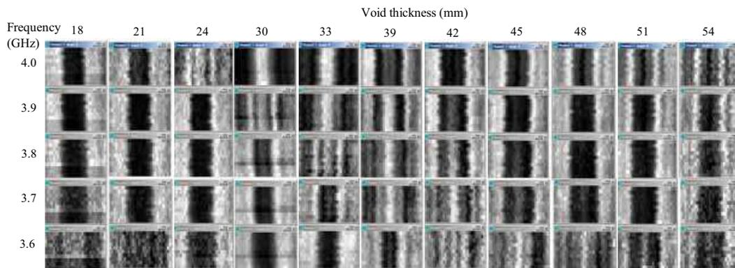
Figure 7: Actual GPR images (Rubber void floor).
