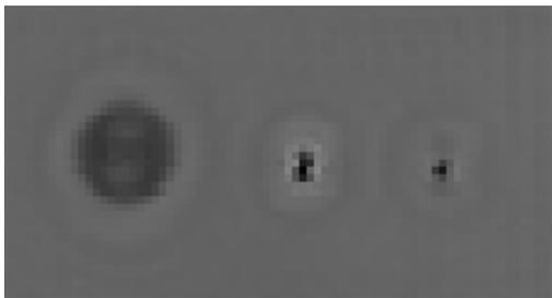
Figure 1: RASCAN subsurface holographic radar image, 3.6 GHz, parallel polarization.
