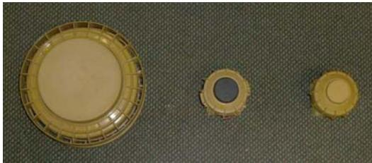
Figure 2: Three plastic body mines; VS-1.6 ( $\Phi=242$  mm), VS-50 ( $\Phi=90$  mm), TS-50 ( $\Phi=90$ mm).
