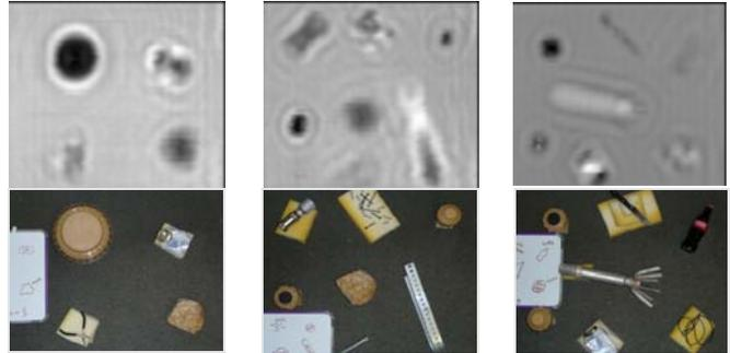
Figure 3: Top - example RASCAN images (75x65 cm); Bottom - matching object layouts as buried in test bed.
