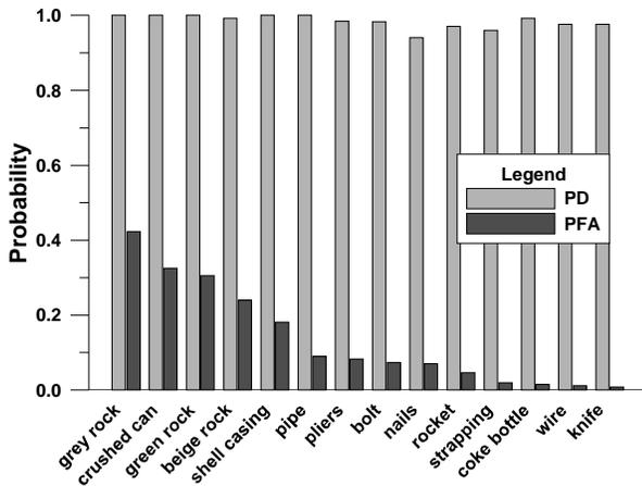
Figure 5: Detection and false alarm probabilities for clutter items.
