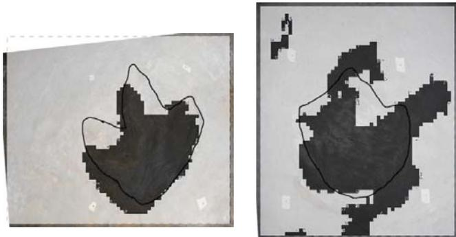
**Figure 7: Binary radar image overlaid on photograph of exposed track (left), and filled track (right). Images are 65cm x 55cm. Colors are 50% transparent “white” and 100% transparent “black”.**
