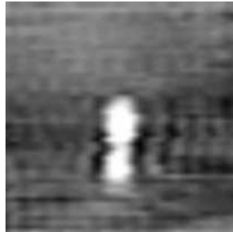
Figure 6: Holographic radar image of a damp cloth between the plastic foam and aluminum sheet.
