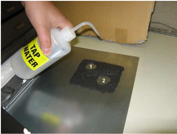
Figure 8: Part of aluminum sheet was covered with glue. Two spots inside were without glue. One of the spots (2) was filled with water.
