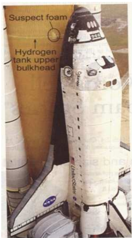
Figure 1: Suspect flaws on the external hydrogen tank coating [1].
