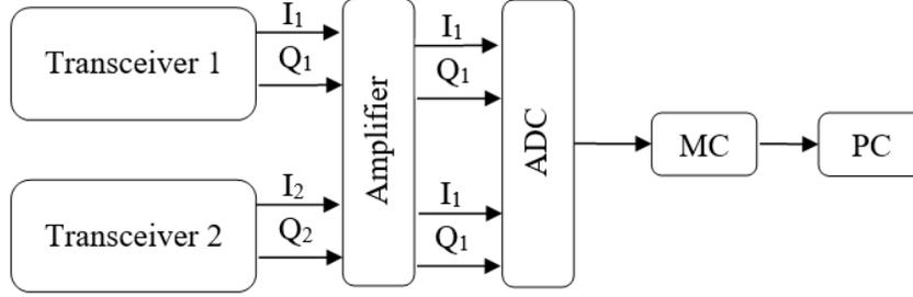
Figure 1: The scheme of the bioradar
